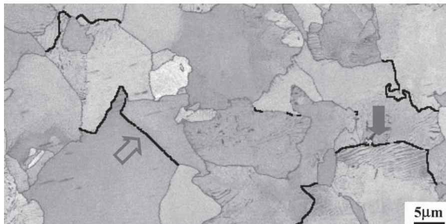
Figure 7 Detailed locations of \Sigma_3 boundaries. (OIM map of specimens heated at 880°C for 33 min and cooled at 10°C/min with the 14 T magnetic field. The magnetic field direction and hot-rolling direction are vertical in this picture. Solid arrow: pearlite boundary; hollow arrow: proeutectoid ferrite boundary. Step size: 0.15 \mu\text{m} .
